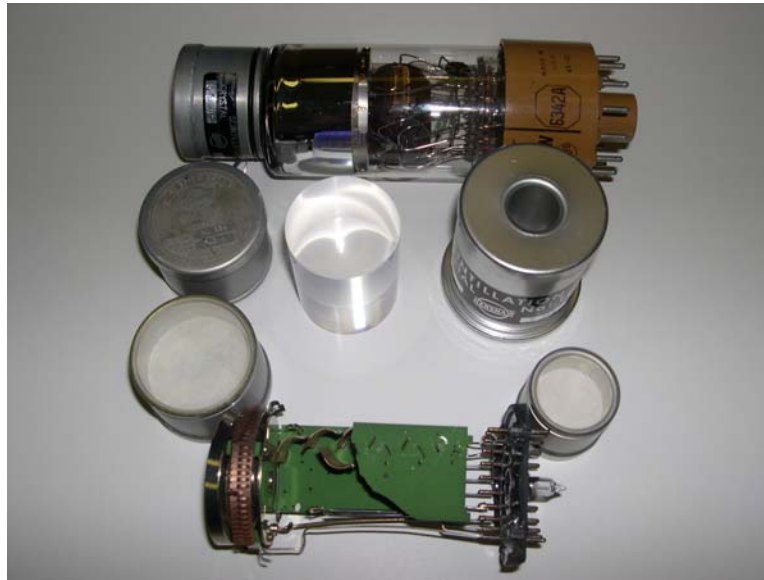
Figure 4. A picture of a photomultiplier tube, several examples of NaI and plastic scintillators and, the insides of a photomultiplier tube showing the curved dynodes.
